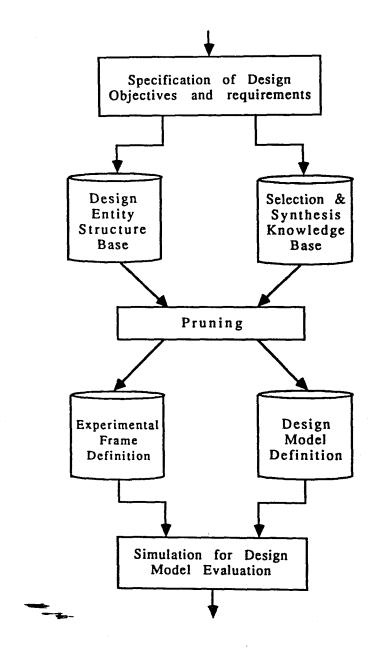
Figure 1 Model-based system design process
